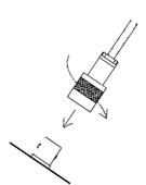
The detector cable can be a source of problems. Test the detector cable by bending or flexing either end of the cable and checking for an increase of counts detected. Replace the cable if increases in the rate of counts are detected.
