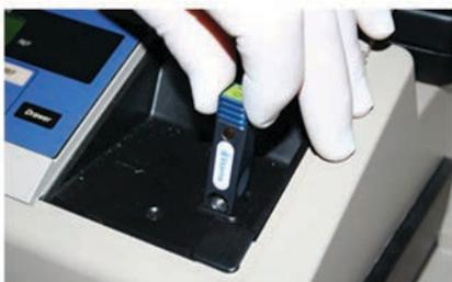
8. Place the DMV-Bio Cell in the spectrophotometer and proceed with the analysis.
