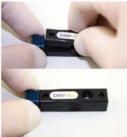
5. Assemble the DMV-Bio Cell by holding down the sample half on the plate and carefully bring the other half in close proximity, such that the bottom of the cell touches first and then gently allows the two halves to come together, preferably without snapping shut.
