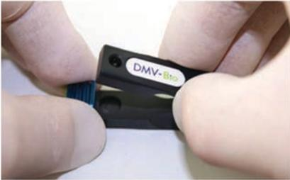
1. Open the DMV-Bio Cell carefully by separating the two halves.
