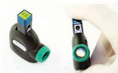
7. Before putting into the spectrophotometer a check for dust or minute bubbles can be performed in the free sample viewer accessory provided.
