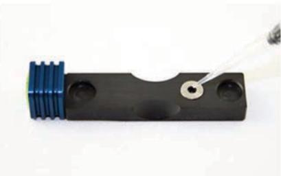
4. Carefully pipette the correct volume of sample to be measured into the sample well in the centre of the ring as shown.
