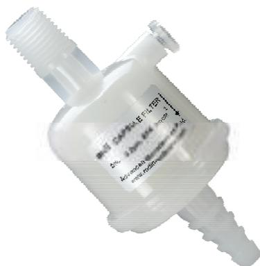
**mdi** 1" AseptiCap NL capsule filters employ Nylon-66 membranes for wide chemical compatibility. These large area filtration devices are ideal for large volume (5 - 20 liter) filtrations such as mobile phase filtration for preparative HPLC and for large laboratories with many HPLC systems.
