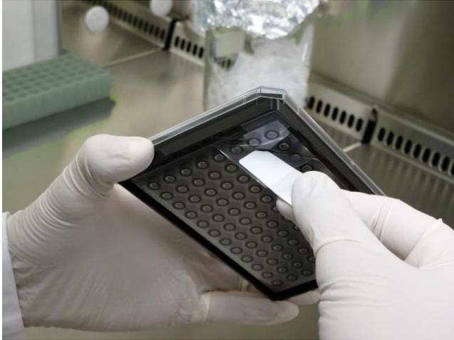
**Fig.4: Pull off the protection foil.**
